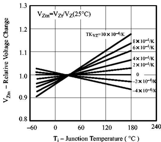
Figure 3. Typical Change of Working Voltage vs.
