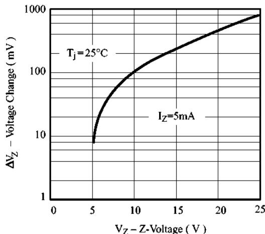
Figure 2. Typical Change of Working Voltage
