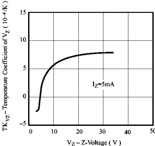
Figure 4. Temperature Coefficient of Vz vs.
